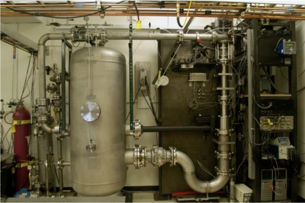
Figure 3-1: Aerospace Corporation's inducer test facility [6]
